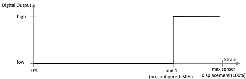
Figure 4: Digital output signal vs. displacement.
